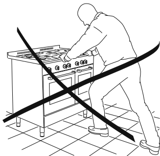
Figure 7 Incorrectly moving the cooker
